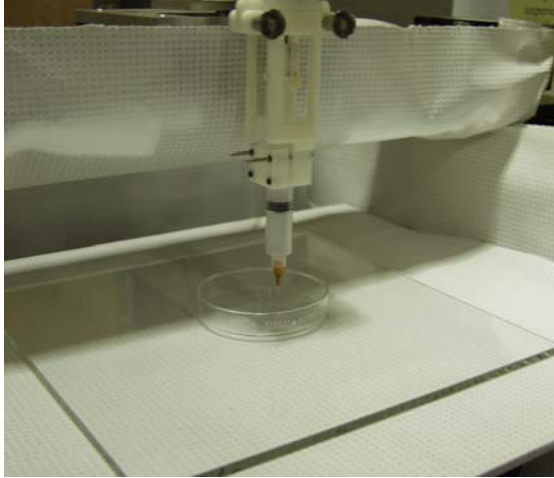
Figure 11 - Isometric View of Deposition Tool and Printer Before Printing Into a Petri Dish
