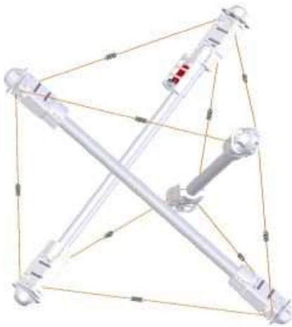
Figure 5: CAD model of a complete modular tensegrity robot
