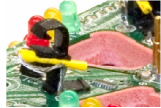
Figure 6. Mechanical latch with an SMA actuator.
