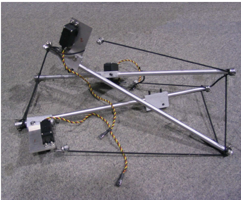
Fig. 7. A robot resembling TR-3 implemented in the real world.
