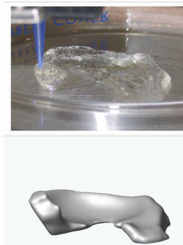
Figure 5. (top) Alginate hydrogel tissue structure being freeform fabricated; (bottom) target geometry, derived from CT scan data
